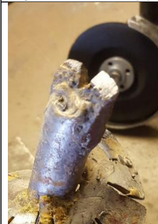
Photo 19. Open the tip in the middle and grind in the right way, like this
