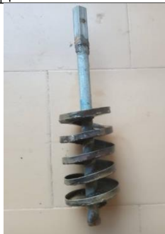
Photo 24. Spiral auger with strips
