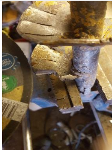
Photo 17. Grind the cutting edge
