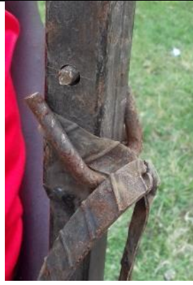
Photo 2. Fast fix pin. If too long there is danger of getting stuck
