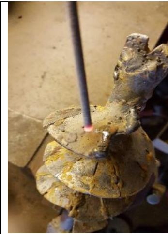
Photo 16. Make cutting edge, weld a rim. (1/2" pipe)
