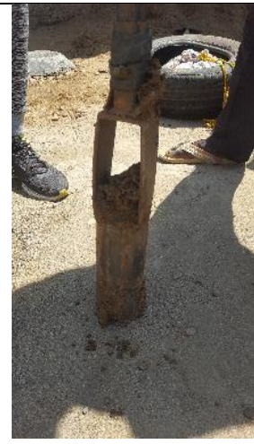
Photo 38. The punch can be cleaned with the Clean pin
