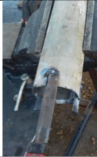
Photo 11. The cutting teeth made with a piece of a flat or half round file.
