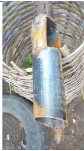
Photo 37. This model uses a tungsten tip. Note the position of the tip.
