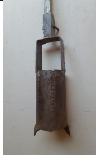
Photo 12. Note that teeth stick outside in a way that the cutting edge is outwards
