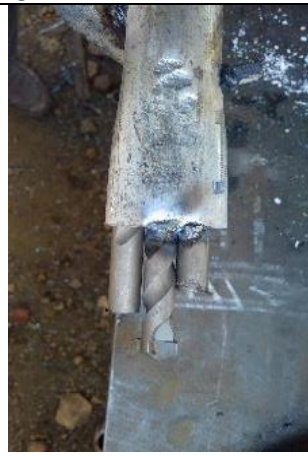
Photo 20. Eventually you can make the tip with a stone drill of 8 mm
