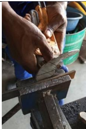
Photo 14. Bend the plate in a vice until opening is 40 mm or more.
