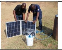
Solar pumps 24 - 35 VDC Pump head 1 pump: 3 - 14m Pump head 3 pumps: 40 m Pump volume 1 p.: 5 - 30 l/min Cost 1 pump set: \$150 – \$250
