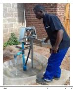
Rope pump 4 models Models for hand dug and hand drilled wells. Cost/pump: \$60 - \$120
