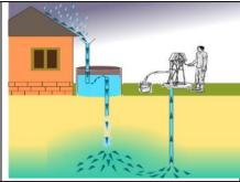
**Tube recharge** Prevents dry wells. Can recharge 100-200 cubic meters /yr. Cost material: \$10 - \$50
