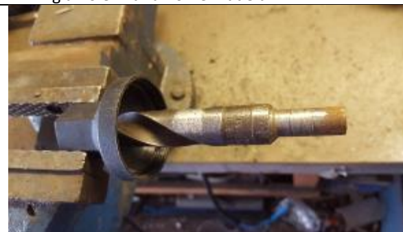
The holes can also be made with a drill bit 13 or 15 mm
