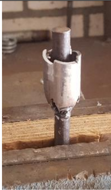
You can drill a hole of 15 mm with a home made drill
