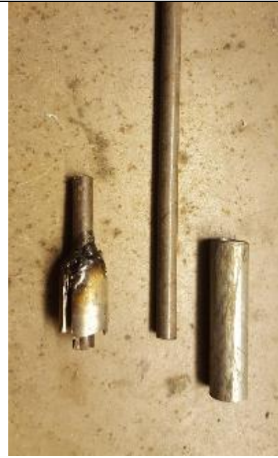
Materials needed; round bar 8mm, pipe of 15 mm
