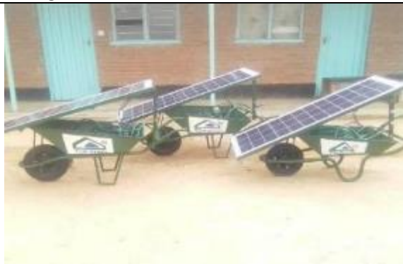
A wheelbarrow pump. A pump, panel, hose and cable mounted on a wheelbarrow. It is easily transported to distance fields for irrigation
