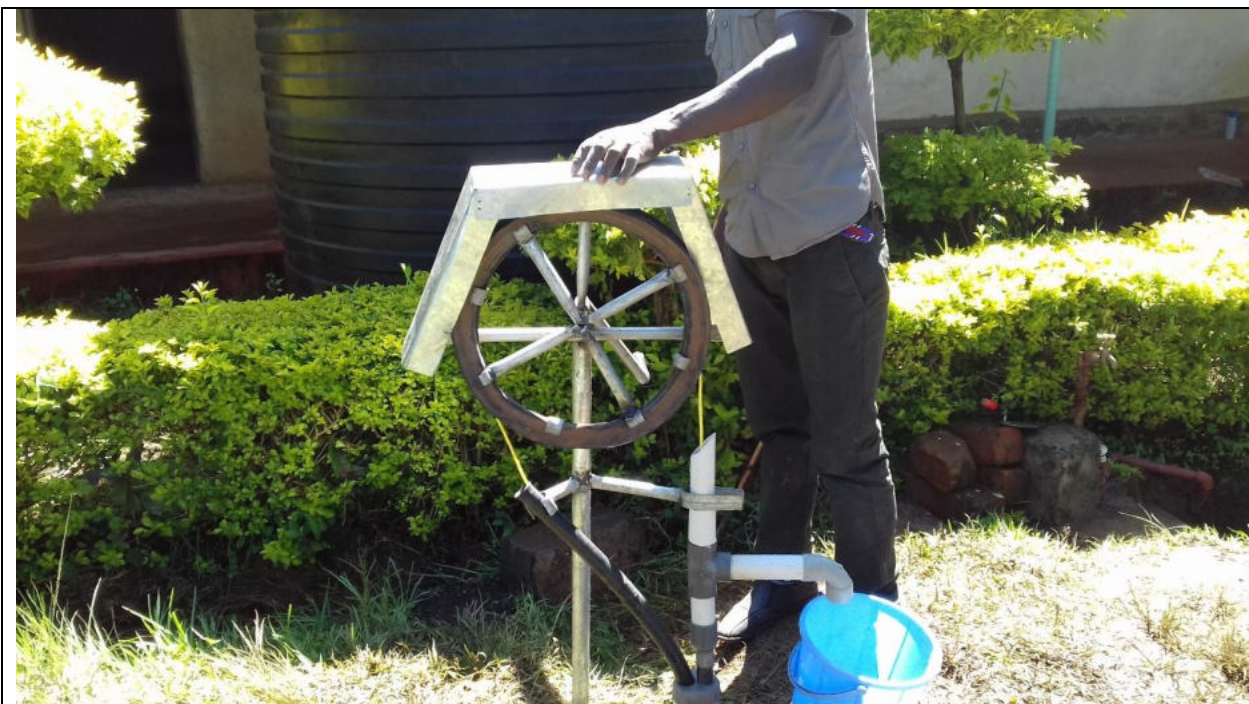
Rope pump with a fixed wheel cover. Note that PVC T piece should be against the outlet pipe support.
