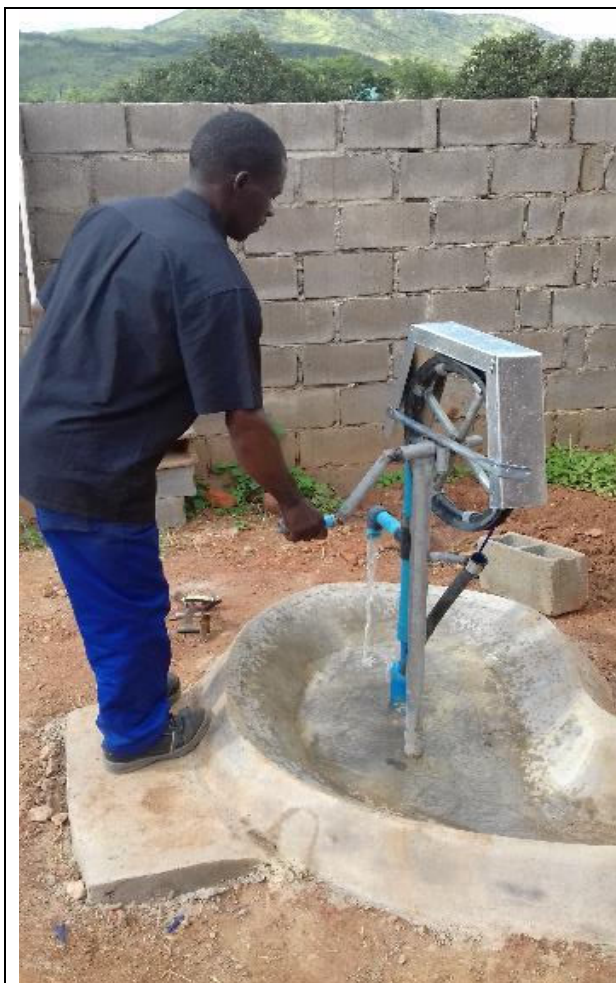
Rope pump model 4 Pole of GI pipe 1¼".
