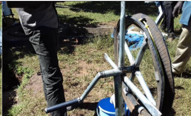
Make sure that the vertical support does not cover the oil hole
