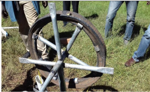
Model with a fixed wheel cover, so with cover supports welded to the frame
