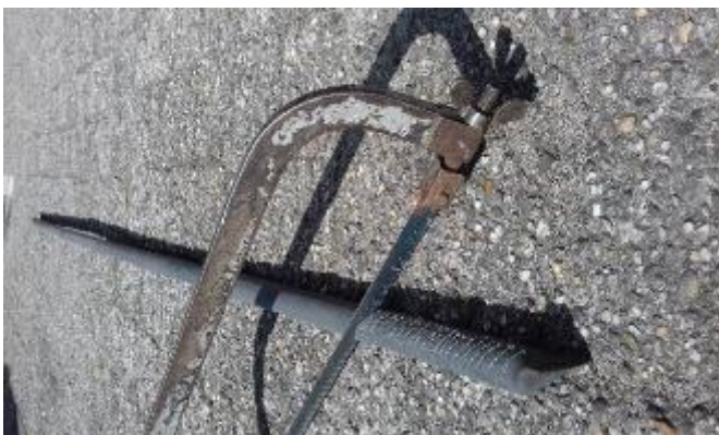
PVC pipe of 3/4" and 3 meter length. Ends are closed. Each side has 0.5 m or more length of slots made with a hacksaw.
