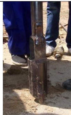
Photo 10. Empty the stone punch with the 2 clean pins
