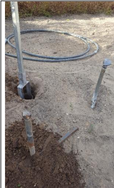
Photo 3. Position of cleaning pins, Left pin 1. On the right pin 2 which has a plate
