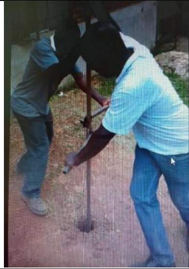
Photo 3. Turn, very slow and push down , to the right until the auger is filled up.
