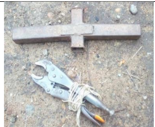
Photo 6. Foot step. Fix Foot step with a Vice grip (Photo) or a rubber strip
