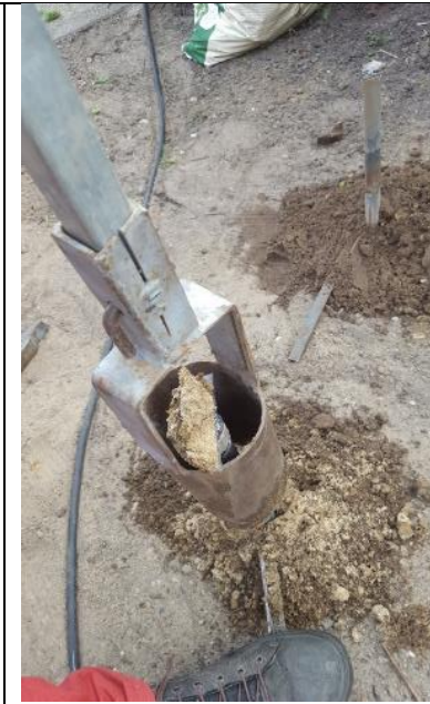
Photo 4. Empty the Auger with pin no 1. If needed with pin no 2
