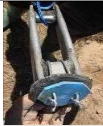
Photo 32. Swabbing tool. In this case attached to a guide box of a Rope pump
