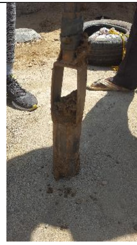
Photo 38. Clean the punch with the Clean pin so push up the soil
