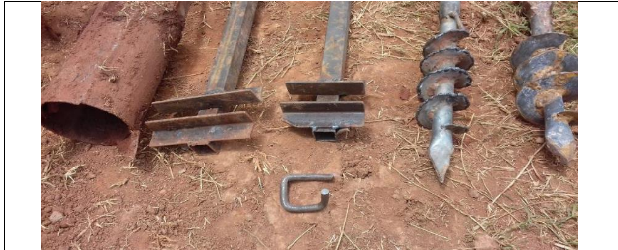
Photo 2. Left; Core auger , 4 inch (4") pipe with inclined teeth to make holes for casings of 4" Middle; Handles , to turn the square drill pipes. Fast fix pin to connect the drill pipes. Right; Spiral augers . A 3" auger to drill a hole for 2 and 3" casings, 4" auger for a 4" casing
