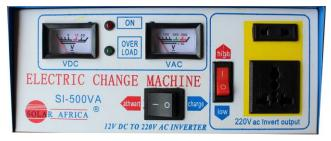
When you are buying such an inverter get one for 400 Watt (Watt=AV) or more and make sure you test the output and choose the one with the highest output voltage.
