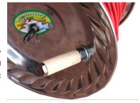
We had to make a reel using two plates (which we normally eat from), a piece of wood, a pipe, a bolt, a few nuts and washers. A screwdriver is used to hold the reel and the bolt to turn it.
