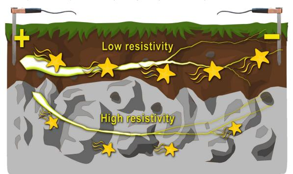
To calculate resistance (in Ohms or  $\Omega$ ), we use the formula Ohms = Volts / Amps. So we need to measure how much current (Amps) is flowing through the soil and we need to measure the difference in Voltage between two points in the soil.
