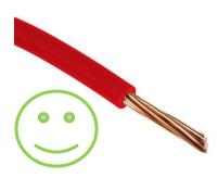
When buying cable, make sure to get stranded wire of 2.5mm<sup>2</sup> (=1.6mm or 14gauge). Wire that has one single core will break easily.
