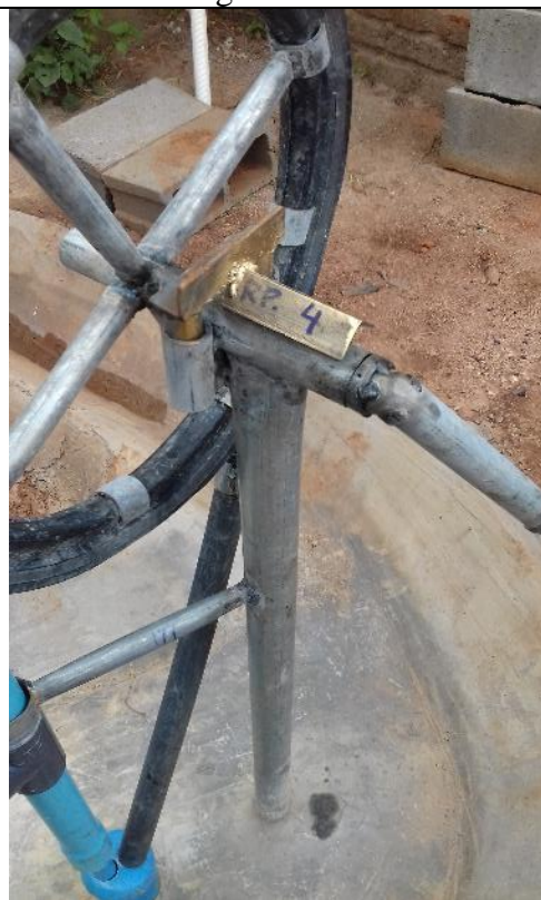
Jig for bushings for wheel support
