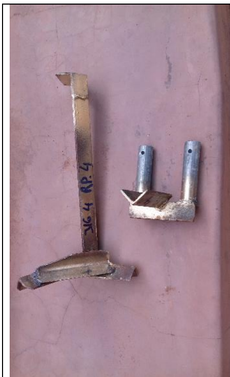
Jigs for position of pipe support and wheel cover mounting
