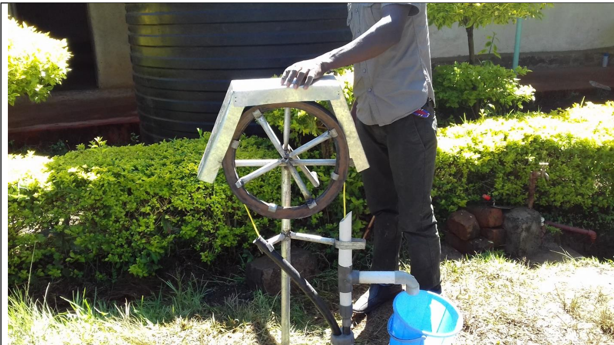
Rope pump with a fixed wheel cover. Note that PVC T piece should be against the outlet pipe support.
