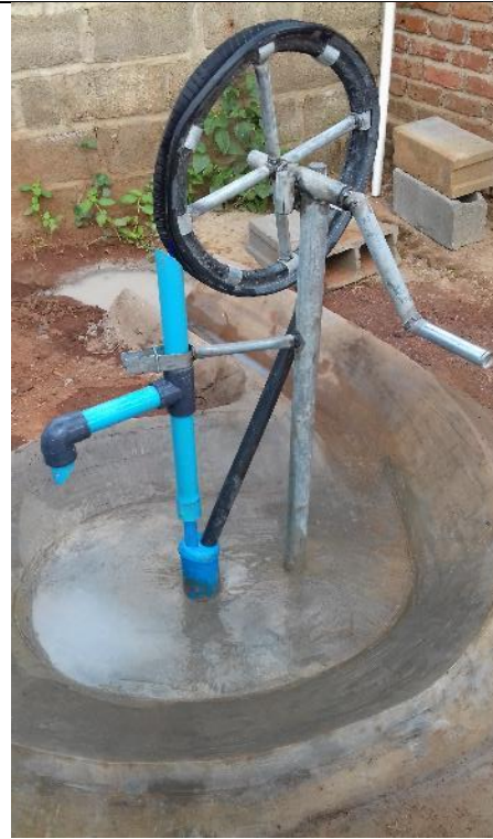
With this model the wheel cover is optional It can be purchased later Pole 0.5 m in the ground / Concrete
