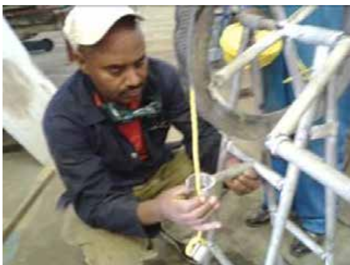
Aligning the outlet support
