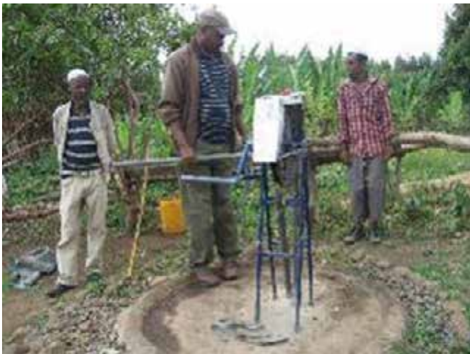
Model 1 Narrow structure, Ball bearings, and Bent legs. Improved model
