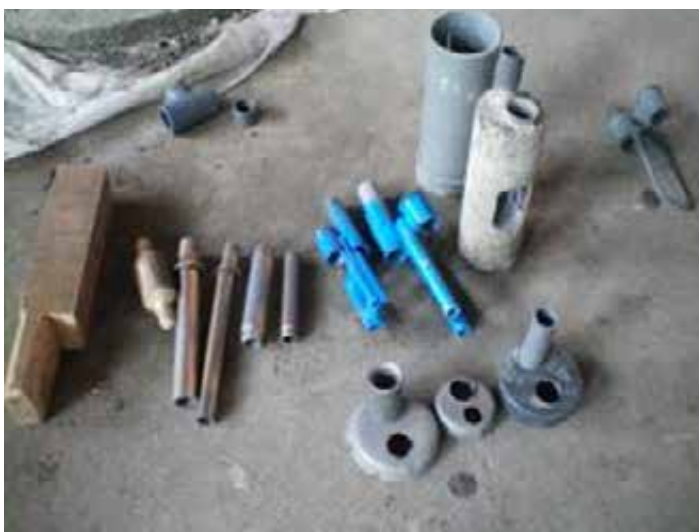
Jigs and tools Incl. socket and trumpet tools, end caps, cement guide block.
