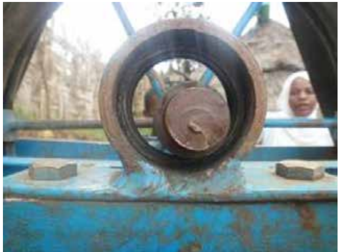
Use of ball bearing but low quality. If ball bearing are used than sealed models with grease nipple
