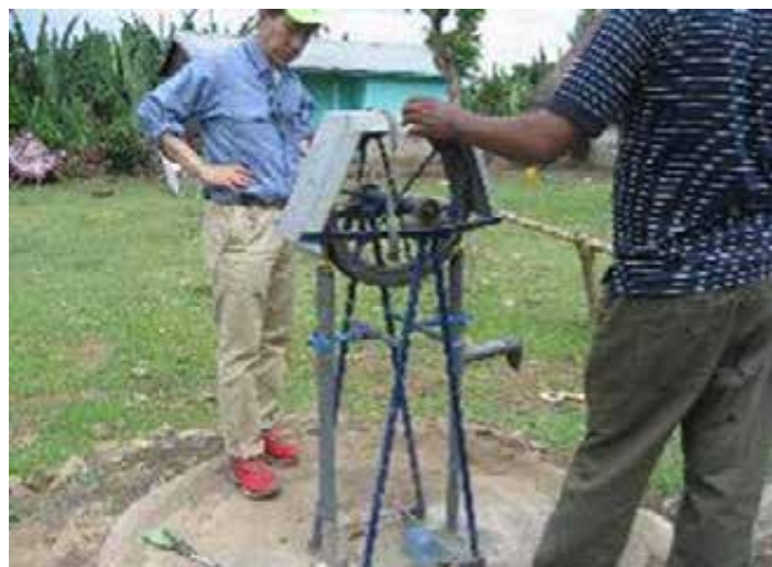
Model 1 Wide structure, Ball bearings, bottom reinforcement. JICA model
