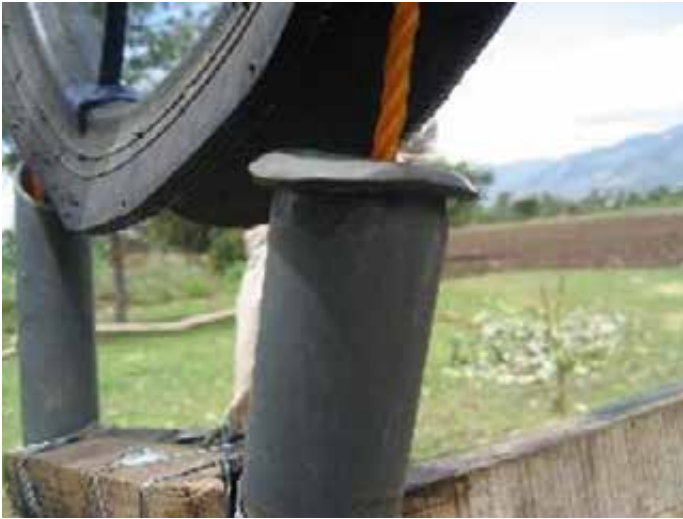
The inlet of the return pipe is not good. It requires a nice smooth entrance, a so called trumpet which can be made with a trumpet tool.
