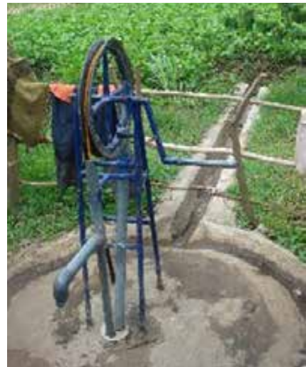
Pump model 2 used for productive use. Here the pumps is used for irrigation of a garden of 300 m2
