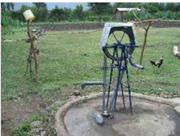
Model 1 Bushings, Bend legs. Pump pipe and return pipe via the 4 inch pipe. Improved model
