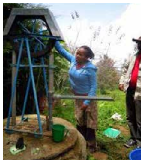
Pump high since it is mounted on a parapet. In this case short base model should have been used or a platform should be installed.
