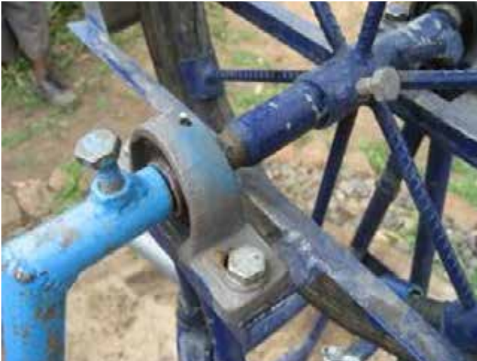
Pump with ball bearings. In this case also supply a grease pump
