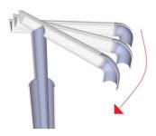
It is advisable not to pump always in the same position of the holder; by varying it, the abrasion of the outlet valve is distributed throughout its surface, thus increasing the valve life span.
