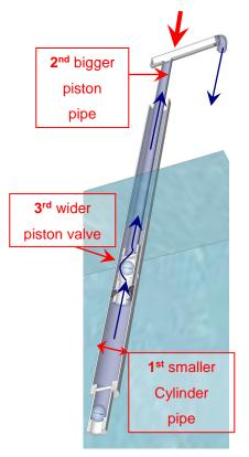
The Pushing motion is easier for human beings then Lifting. The required pushing power depends mainly on friction in piston valve and the piston or pumping pipe. This friction is mainly caused by the speed in which the water is squired through the piston valve and piston pipe.
