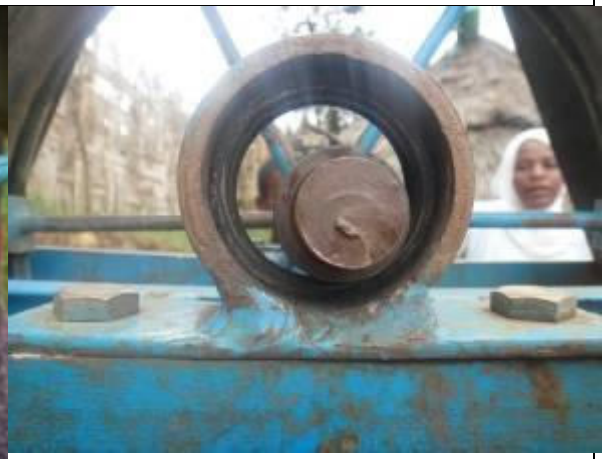
Use of ball bearing but low quality. If ball bearing are used than sealed models with grease nipple
