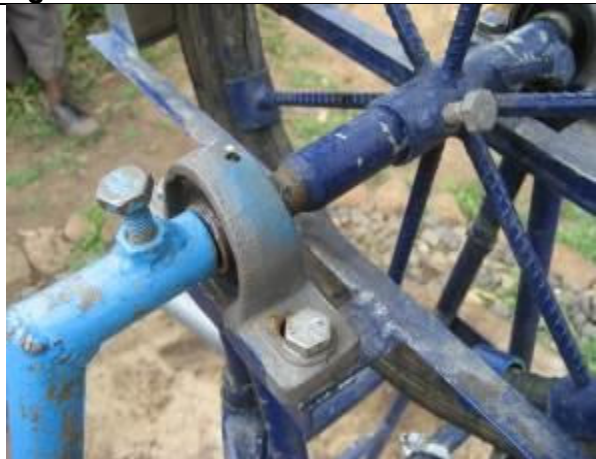
Pump with ball bearings. In this case also supply a grease pump
