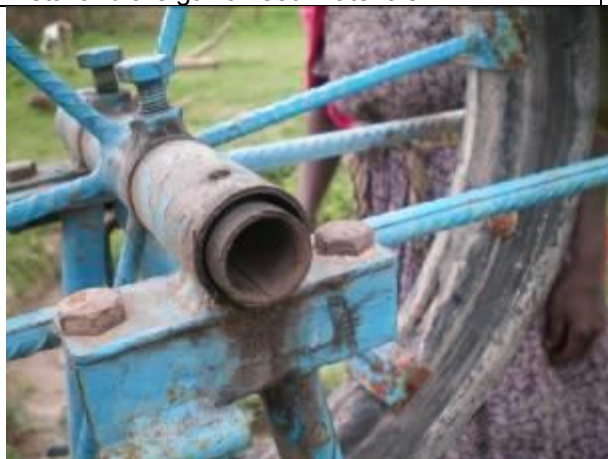
To much clearance in bushing resulting in extra wear
