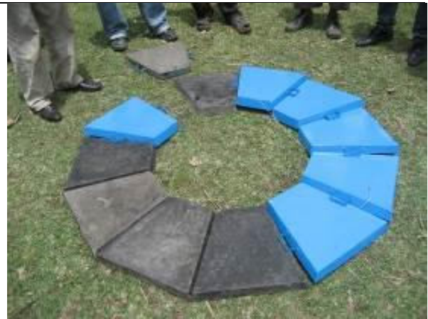
Special tapered blocks to make a well ring
