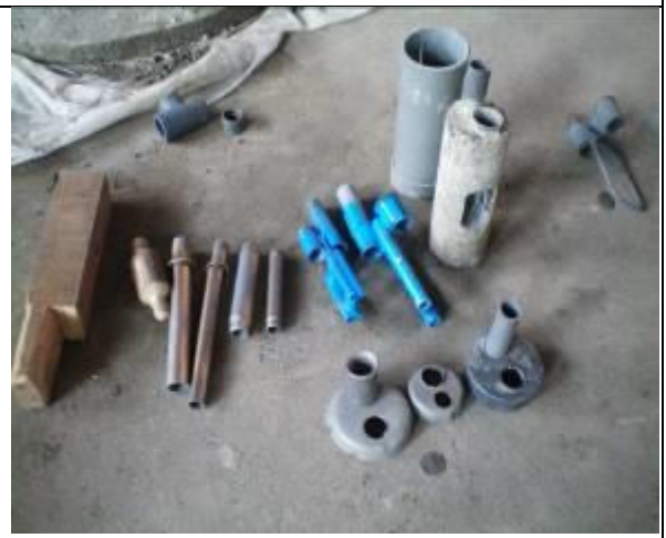
Jigs and tools Incl. socket and trumpet tools, end caps, cement guide block.
