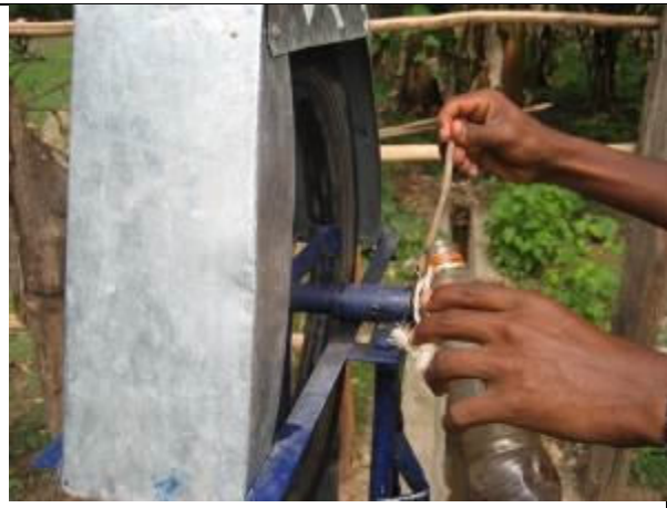
Lubrication of bushings. The oil hole should be on top
