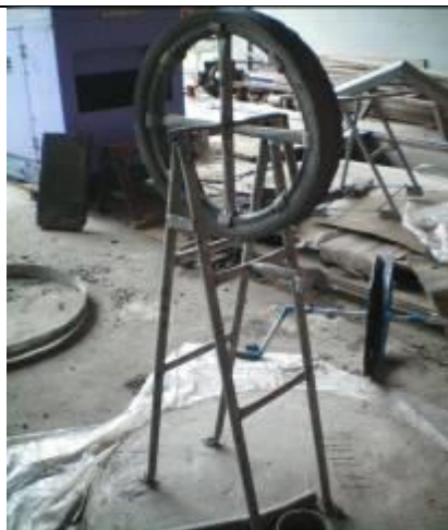
Mounting of Rope pump Model 2. A frame, economy model. Instead of welding angle iron and rebar, legs are bend and have a hole so less material and less welding
