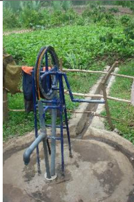
Pump model 2 used for productive use. Here the pump is used for irrigation of a garden of 300 m2
