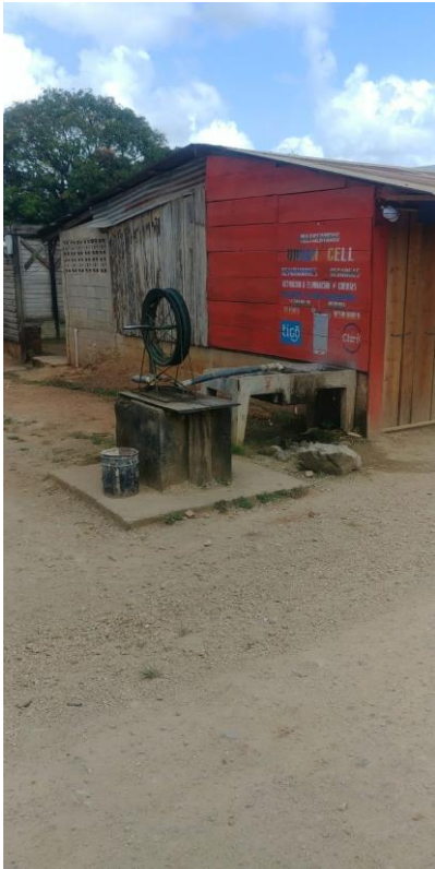
Photo 14: Functioning rope pumps on family hand dug wells in urban area (Rosita, RACCN).
