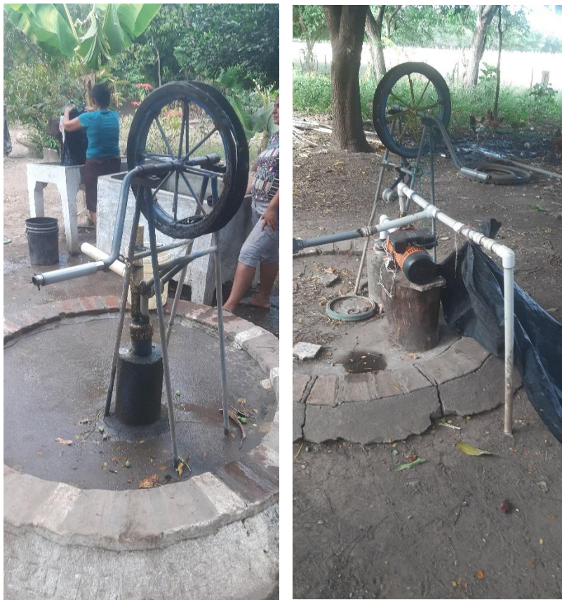
Photos 7: Original rope pump still in use, Matapalo village, Municipality of Villanueva, Chinandega.
