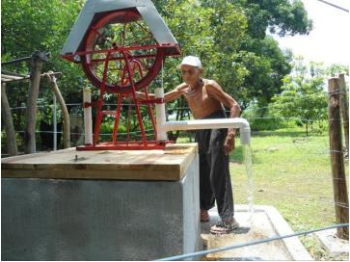
Photo 2: Standard rope pump manufactured by Bombas de Mecate, S.A. (BOMESA), El Cedro.
