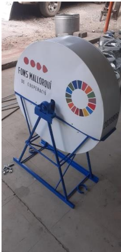
Photo 4: Standard rope pump with protective covering made by Fabrica de Artículos Metálicos , Somoto.
