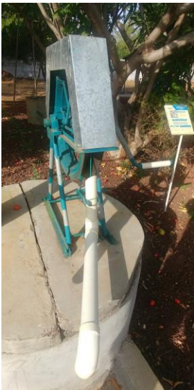
Photo 3: Standard rope pump manufactured by AMEC, Managua. This model uses galvanized pipe, wheel cover and a smaller wheel
