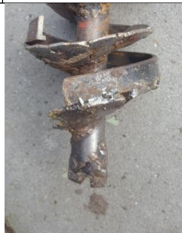
Photo 23. You can increase the lift capacity by welding a 15 mm strip around the plates
