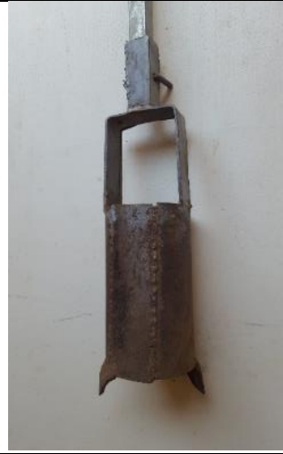
Photo 12. Note that teeth stick outside in a way that the cutting edge is outwards
