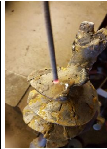
Photo 16. Make cutting edge, weld a rim. (1/2" pipe)
