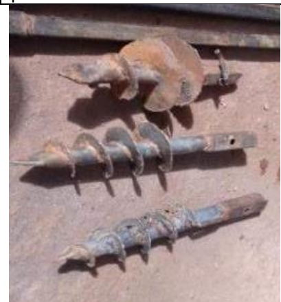
Photo 21. To increase the capacity you can bend up the plates
