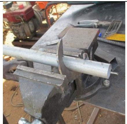
Photo 15. You can also bend the plate by welding it on the pipe and hammer it. Here the pipe is 3/4" GI
