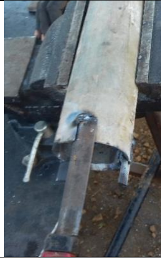
Photo 11. The cutting teeth made with a piece of a flat or half round file.
