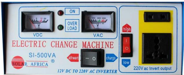
When you are buying such an inverter get one for 400 Watt (Watt=AV) or more and make sure you test the output and choose the one with the highest output voltage.
