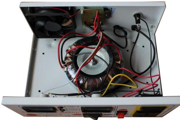
Also the inverter needs to be of an old generation using a coil and not mush electrical components because they are more robust for our type of work. Some of these inverters have a high out put switch, good for us.
