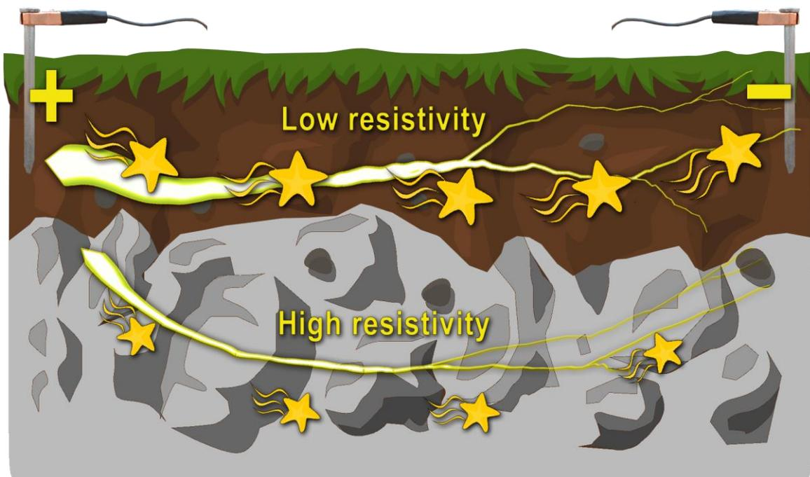
To calculate resistance (in Ohms or  $\Omega$ ), we use the formula Ohms = Volts / Amps. So we need to measure how much current (Amps) is flowing through the soil and we need to measure the difference in Voltage between two points in the soil.
