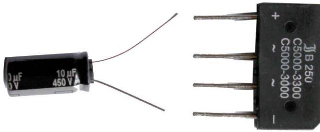
To make DC from AC, use a bridge rectifier (4 pins) and a capacitor of 1 µF suitable for 400 Volt or more. These components can be found in old heavy TV's or buy them online.
