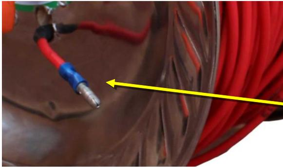
We made relatively long wires sticking out of the witch box. This is done so that the reels can be laying on the ground while the switch box is on the “working table” or suitcase. There is no long wire sticking out of the reel because it will be in the way when rolling it.
