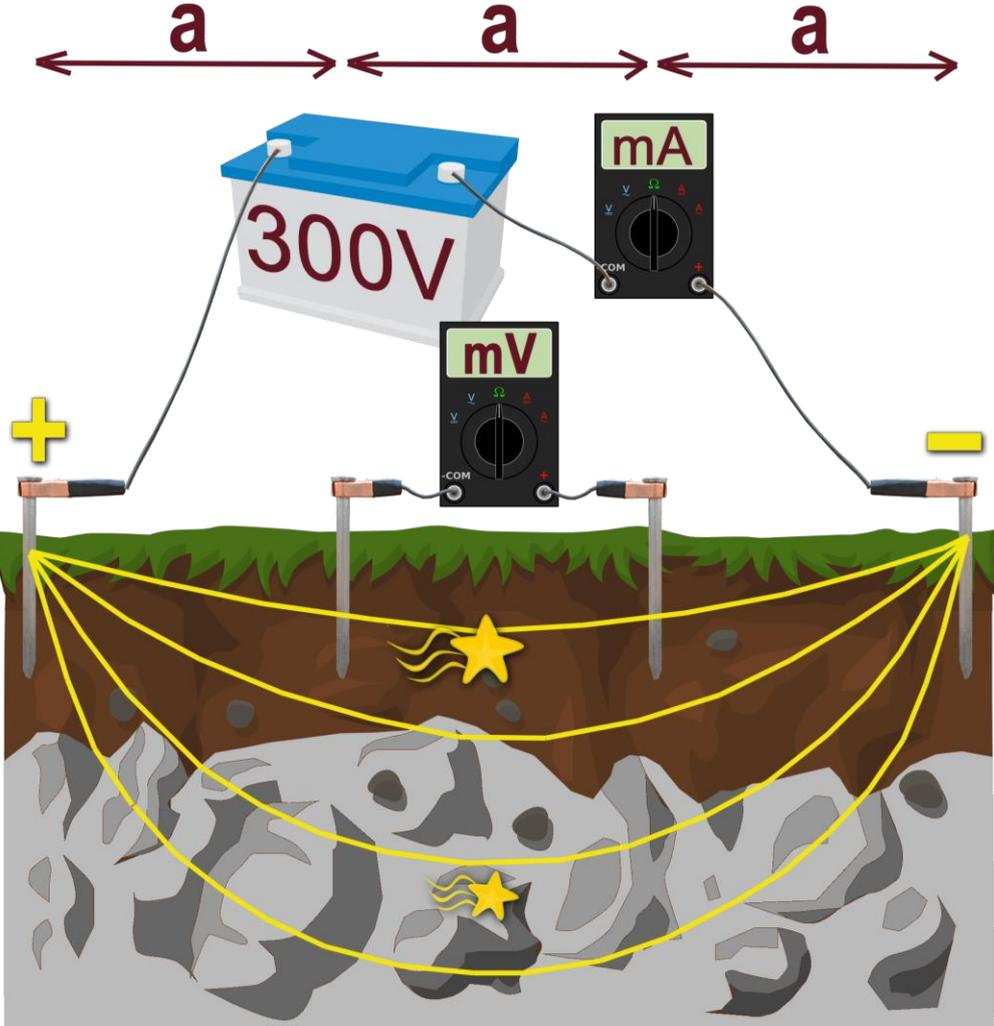
Note: this is a theoretical sketch; in reality, we will use a normal 12V battery with an inverter and a rectifier to generate 300V DC.
