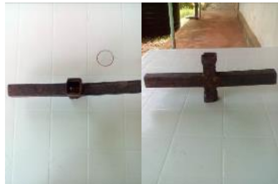
Foot step. In case rubber strips are used instead of a Vice grip, weld strip to avoid cutting of the rubber strip
