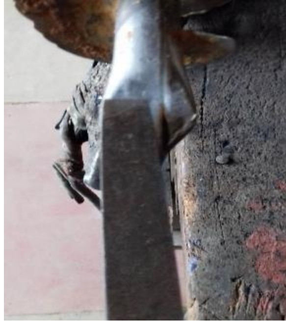
Make the point flat. Weld a piece of an old flat file on the point. Sharpen with and angle grinder, make a cutting edge.
