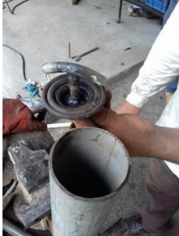
Combi bailer 3 inch. Valve made of Round bar 10 mm. Outside diameter .. mm. And a plate of 3 mm
