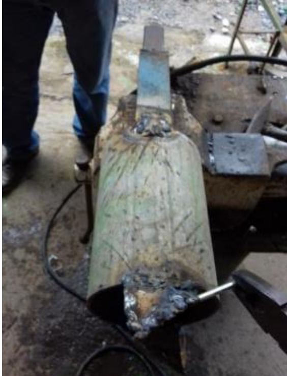
Core Auger 4 inch. The teeth can be made by cutting and welding an extra piece reinforced with a hard materials like a file. Here the tip is a 6 mm concrete drill bit with tungsten tip
