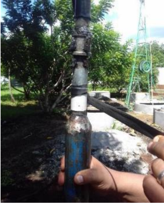
To make it a closed bailer push down the PVC pipe.
