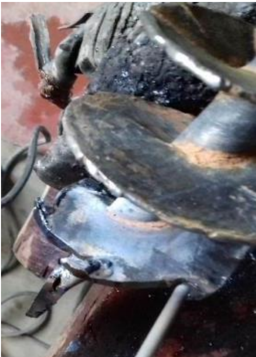
Eventually make teeth on edge of the plates Weld a spot and grind a teeth. Note the cutting edge of the point
