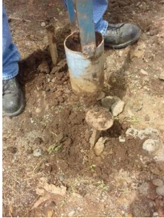
The second step is cleaning with second pin, a pin with a plate of 8 cm round that fits inside the core auger of 5 inch
