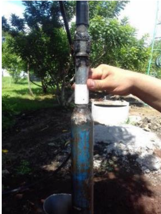
Open the bailer in case of deeper wells and soils with coarse sand or gravel In closed position the bailer will work till depth of 5 to 8 meters.
