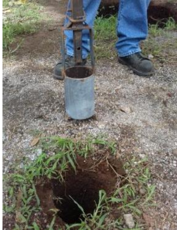
Core auger 5 inch combined with spiral auger inch. This can be used when the soil is to wet to stay inside the Core auger .
