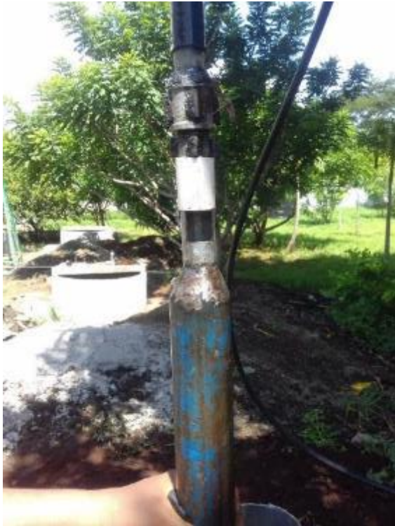
Combi bailer 2 inch. This bailer can be used in closed and open position. In this case it is in an open position.
