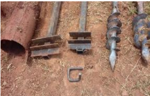
Handles. These are made of square pipe and angle iron of 25 mmx 2.5 mm. or the same square pipe. See last page
