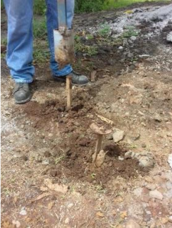
Cleaning pins. The core auger can be cleaned by pushing the core auger on the small cleaning pin
