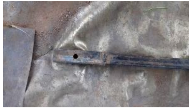
The connections. made of square pipe 32 mm with 1.6 mm wall thickness
