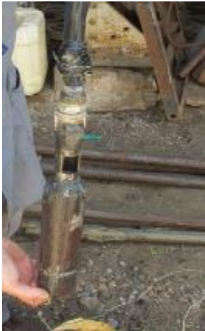
Make an opening at the top of the bailer Weld 2 pins at the lower end. (Pins can be for example the axle of a bike front wheel) Make sure bailer fits in the used casing with min 10 mm clearance.
