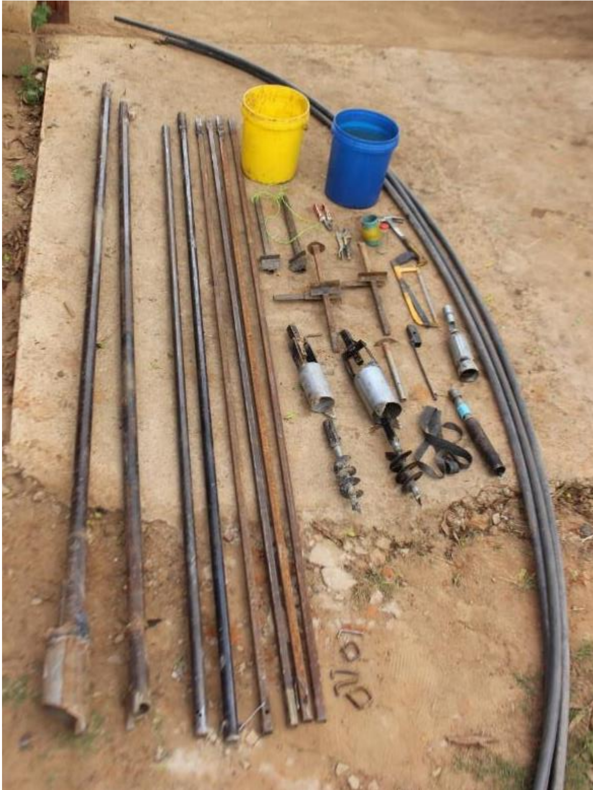
A Mzuzu drill set . In this picture the set is for wells to 12 m deep.
