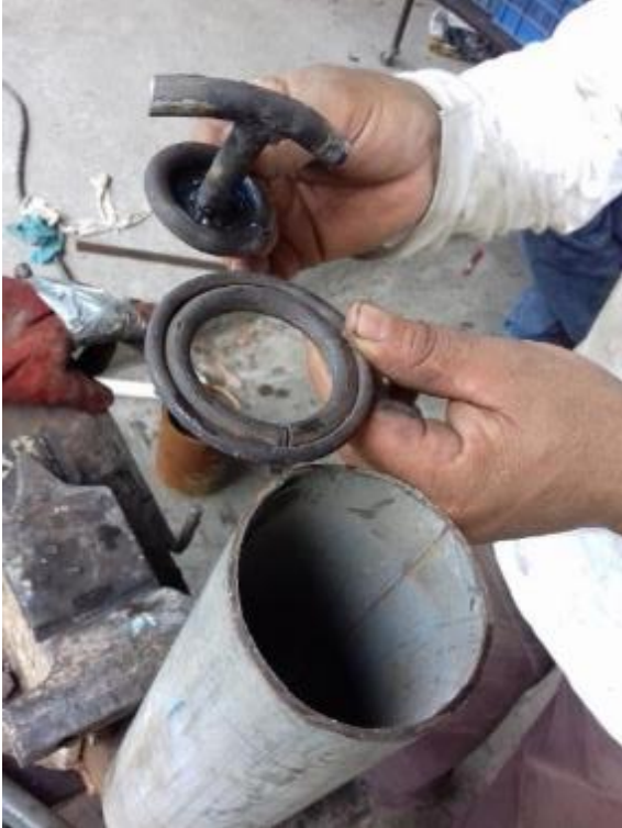
Combi bailer 3 inch. Production of a 3 inch bailer. Valve seat made of round bar 10 mm and 6 mm
