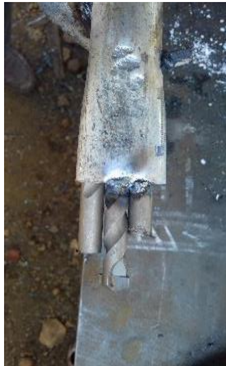
Use a 8 or 10 mm tungsten drill bit to weld in the tip of the auger. Cut in 3 pieces and grind the edge of the tips on the sides also with an angle
