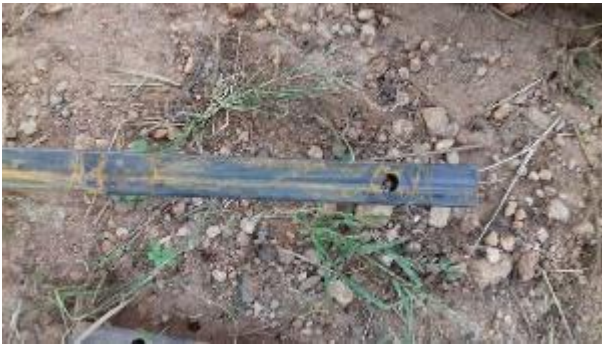
The extention drill pipes. Made of square black pipe of 25 mm. The number of pipes depend on depth. Start with 6 pipes of 3 meter length
