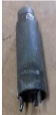
Make an opening at the top of the bailer Weld 2 pins at the lower end. (Pins can be for example the axle of a bike front wheel) Make sure bailer fits in the used casing with min 10 mm clearance.
