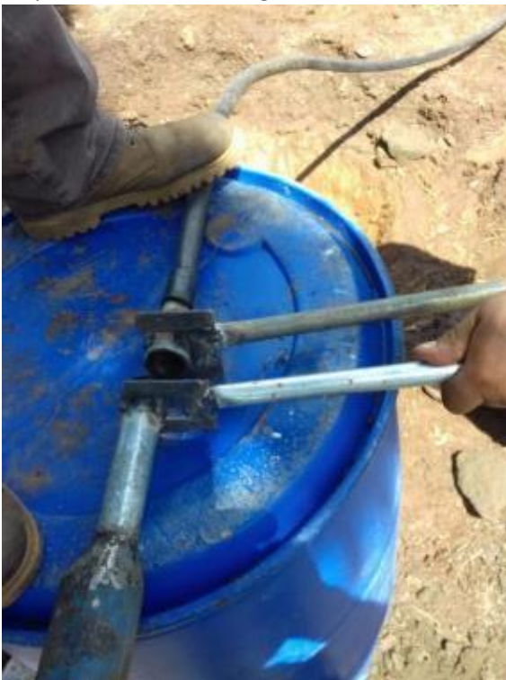
A tool to connect a bailer to the 1 inch Poly pipe/ tube
