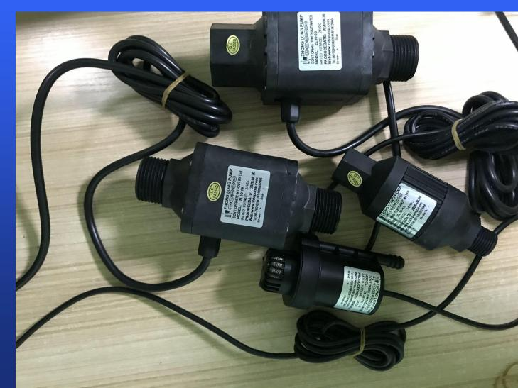
Solar pump. Future pump Capacity: 100 Watt Suction; max 7 m, pressure 10 m Capacity; 15 m head. 3000-5000 ltr day Cost; 700-800 US\$
