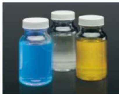
Figure 2: Colilert tubes. Results: colourless=negative, yellow=coliforms, yellow and fluorescent=E.coli
