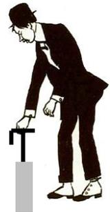
Primary: The more volume you are pumping in one stroke, the heavier pushing will be. So a bigger Cylinder pipe will require more force when pushing the handle down.
