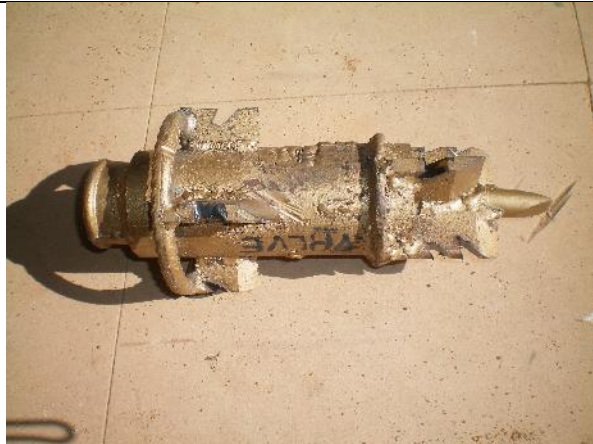
One of the drill bits used for SHIPO drilling. It uses shafts of a bicycle as drill teeth and a 'floating valve' as foot valve.
