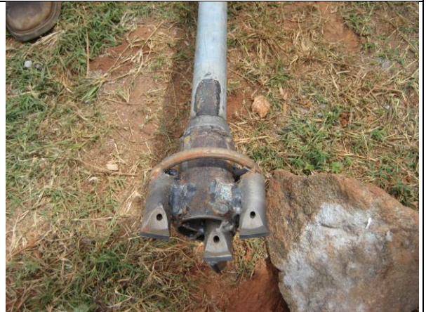
New drill bit using tungsten tips. These drill bits can drill hard layers like sand stone and laterite without getting blunt.
