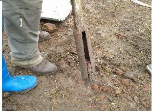
The Soil punch can be emptied by hammering the 2 inch pipe.
